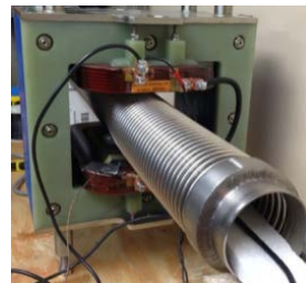
Figure 3: AC Scan Magnet Field Measurements.
