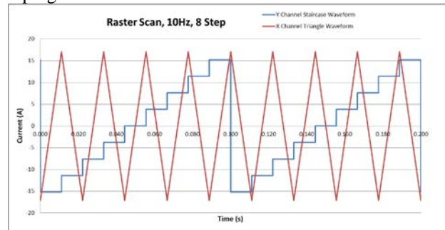
Figure 6: Blue staircase function (10 Hertz) fed to one AC Scan Magnet for vertical component of beam raster scanning, and red triangular waveform (50 Hertz) fed to the other AC Scan Magnet for the horizontal component of beam raster scanning component.
