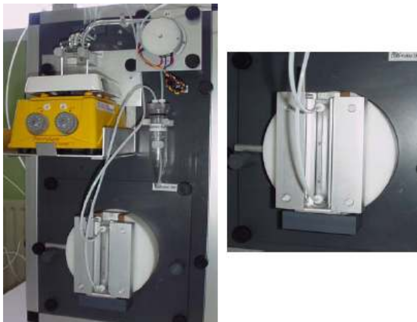
FIG. 7. Manifold for Dissolution and Precipitation of the Target Material. Right Side of the Figure Shows a Close up of the Dissolution Plate Holder
