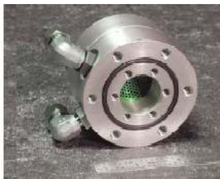
FIG. 7. Picture of ^{18}\text{O} water target from the Pulsar linear accelerator from AccSys. Note the grid covering the front foil to enable front foil to withstand higher pressures and beam currents.
