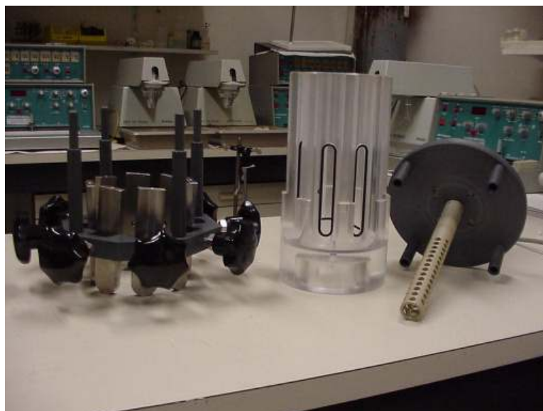
FIG. 3. Bath for production of eight targets simultaneously
