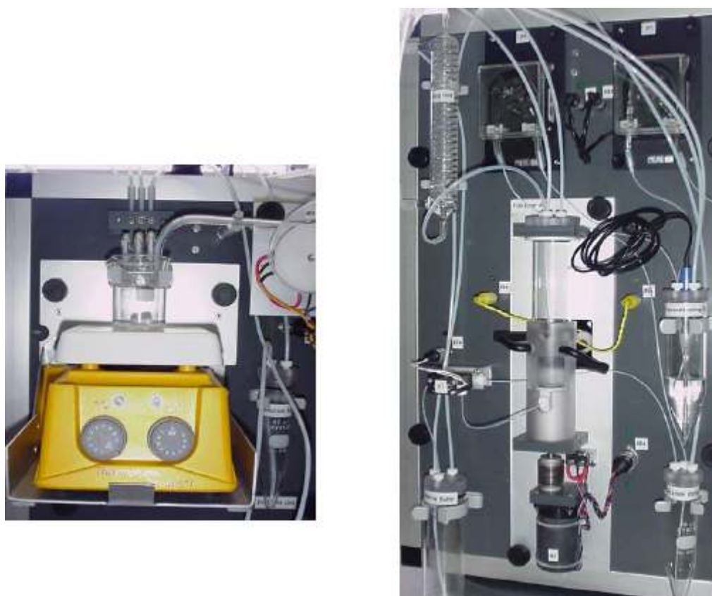
FIG. 8. Manifold used for the precipitation of ^{201}\text{Pb} (left) and the filtration of the final solution (right)
