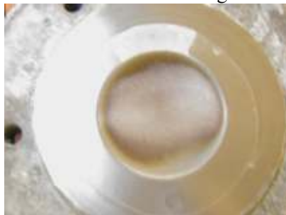
FIG. 4. An example of silver colloid being deposited from solution inside the front foil of a water target
