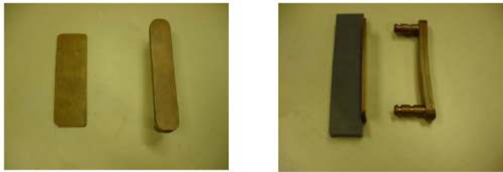
FIG. 4. On the left is the front view of the target carriers and on the right is the side view showing the water cooling connections
