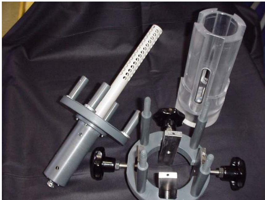
FIG. 2. Plating apparatus for plating four targets simultaneously. The materials of construction are Lucite for the bath and other plastics for the other elements
