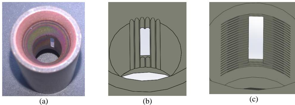
**FIGURE 4.** Surface modification to anode slit area. (a) Anode interior textured with ‘media’ blasting (b) 6 vertical grooves, 0.13 mm deep, (c) 22 circumference grooves, 0.08 mm deep, pitch 0.254 mm
