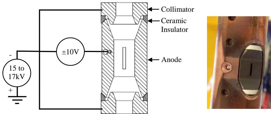
**FIGURE 8.** Plasma electrode – biased anode slit
