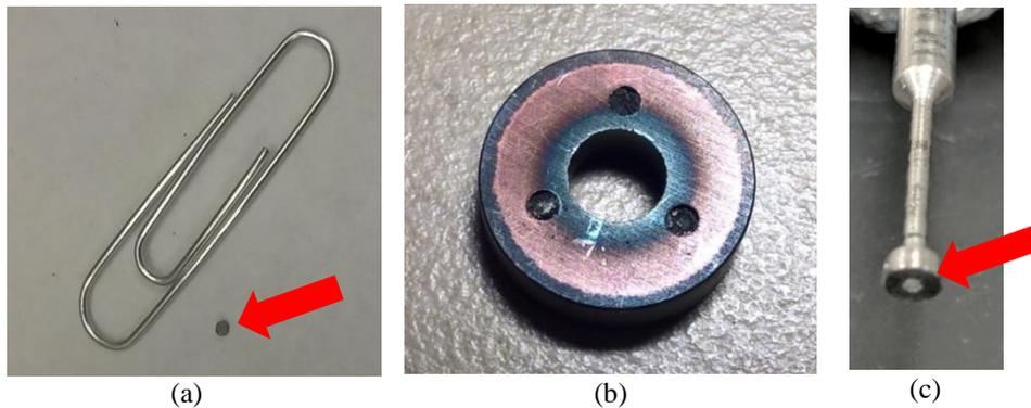
**FIGURE 6.** (a) Cesium getter pill, (b) Cesium getters installed in collimator, (b) Cesium getter installed in cathode
