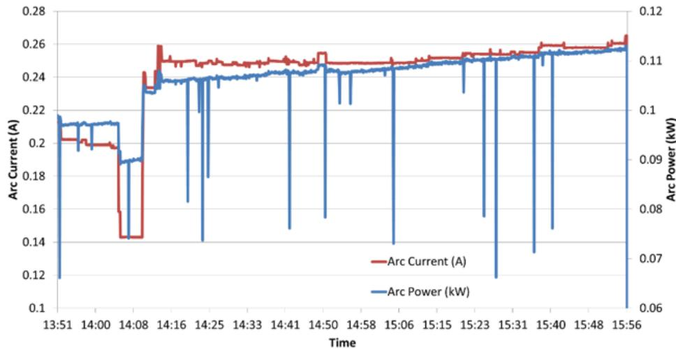
**FIGURE 7.** Following an initial reduction of arc power (-25%) and an increase in beam current (+26%) after cesiation, the arc current and power gradually increased over a two-hour ion source operation (for target beam current controlled to a set point of 150  $\mu$ A by varying arc current).
