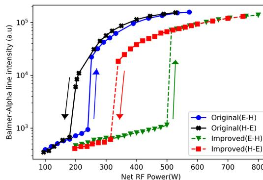
Figure 6: E-H mode transition for original design and improved design(dotted lines) for hydrogen plasma at a gas flow of 10 sccm. The up arrows (E-H) indicate increasing power and down arrows (H-E) indicate decreasing power
