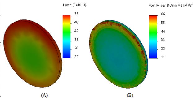
Figure 4: (A) Temperature & (B) Stress distribution on the surface of AlN window that faces the plasma in the improved design for 2500 W plasma power. Other components are not shown.
