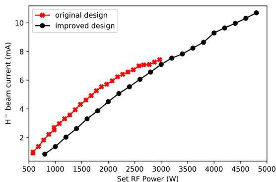
Figure 5: Beam currents achieved for improved design (22 sccm gas flow) and original design [1] (15 sccm gas flow) in H<sub>2</sub> plasma & 30 keV beam energy. Beam current is measured using a Faraday cup placed at a distance of 480 mm from plasma electrode.
