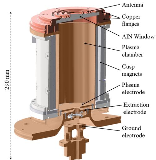
Figure 1: Section view of ion source and extraction.
