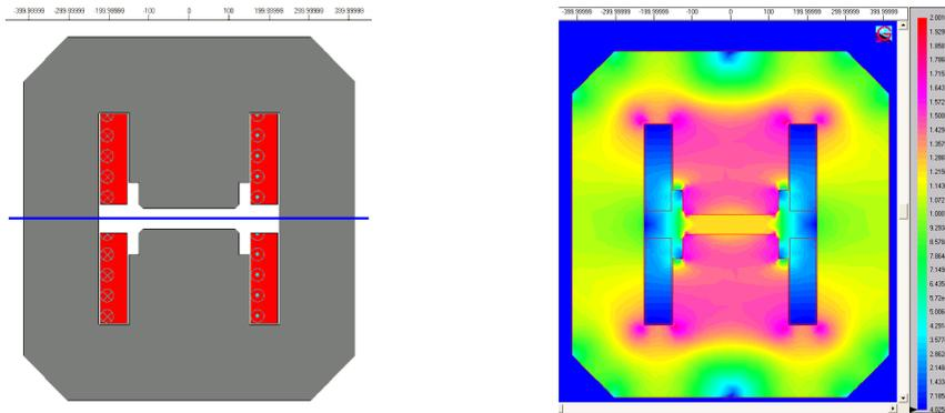
Fig. 3. **Left:** Analyzer Magnet 2D Magnetic Model. **Right:** Magnetic Field as a Function of Colour.  $B_{Max}(0,0,0) = 1.24685 \text{ T}$ ,  $I_{Max2D} = 187.065 \text{ Amps}$ . The central pole is just entering into saturation at  $\sim 1.5 \text{ Tesla}$ .
